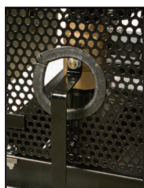
Silent air control with quick position handle
